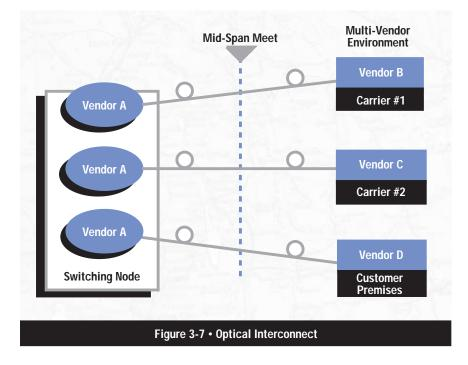
SONET allows optical interconnection between network providers regardless of who makes the equipment. The network provider can purchase one vendor's equipment and conveniently interface with other vendors' SONET equipment at either the different carrier locations or customer premises sites. Users may now obtain the OC-n equipment of their choice and meet with their network provider of choice at that OC-n level.
