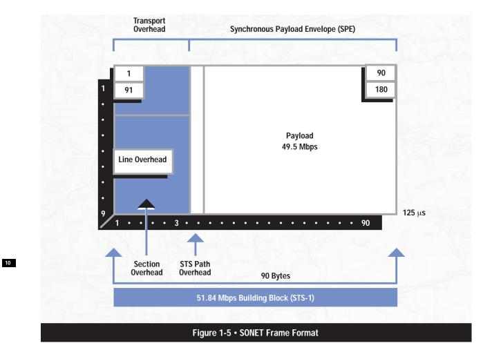
The STS-1 frame format is usually depicted as a matrix of nine rows of 90 bytes each as shown in Figure 1-5. The signal is transmitted byte-by-byte beginning with byte one, scanning left to right from row one to row nine. The entire frame is transmitted in 125 microseconds.
