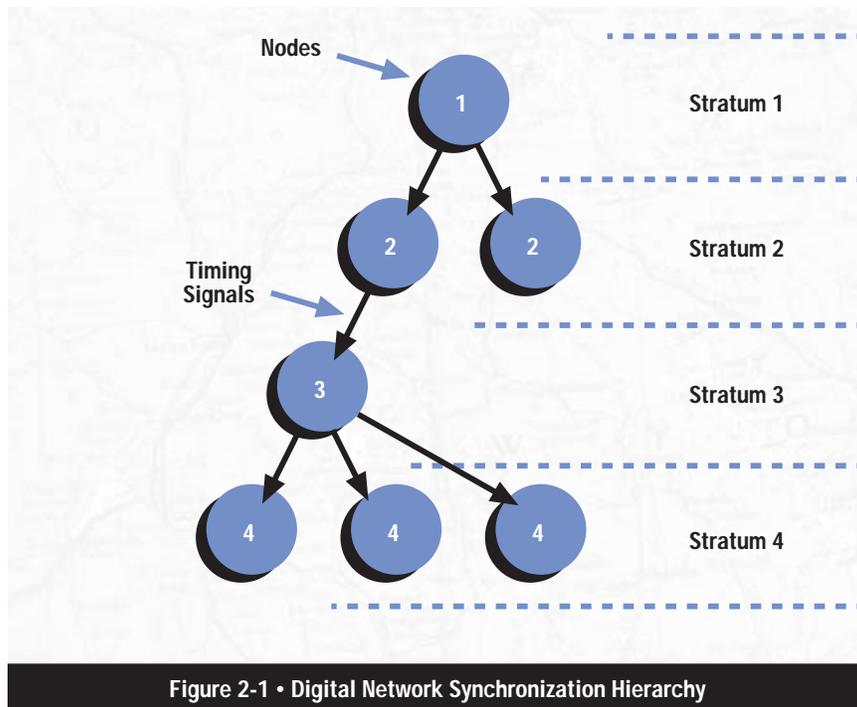
Figure 2-1 • Digital Network Synchronization Hierarchy
