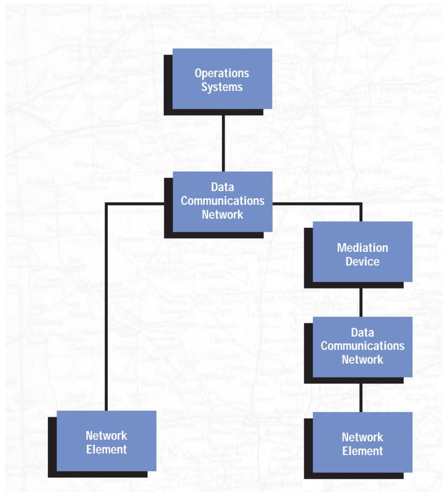
Figure 4-3 • Telecommunications Management Network OAM&P Communications
